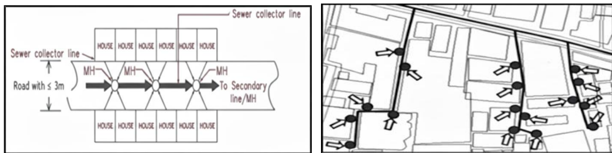
Figure 2: Conventional (Left) and Non-conventional (Right) Sewerage Connection
