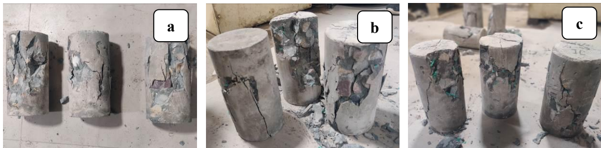
Figure 6: a) PC, b) RPFRC-0.5, c) RPFRC-1
