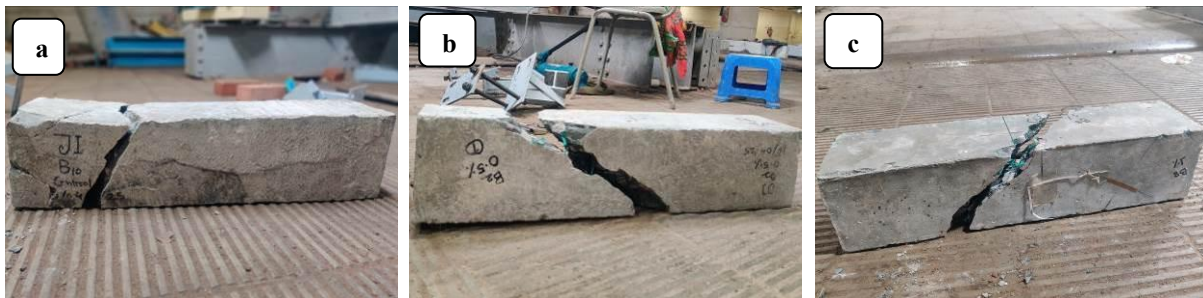
Figure 13: Torsional crack patterns for a) PC, b) RPFRC-0.5, c) RPFRC-1
