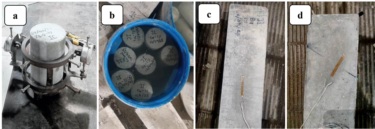
Figure 3: a) Installation of compressometer, b) Curing of cylinders, c) Strain gauge for flexural test, d) Strain gauge for torsional test
