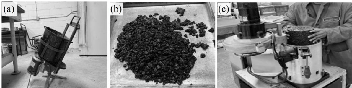
Figure 3: Sample preparation: (a) Mixture machine, (b) Mixed aggregates and (c) Sample through gyratory
