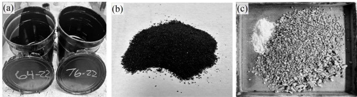
Figure 1. Materials used in the study: (a) Asphalt binders, (b) Ground Tire Rubber, and (c) Aggregates
