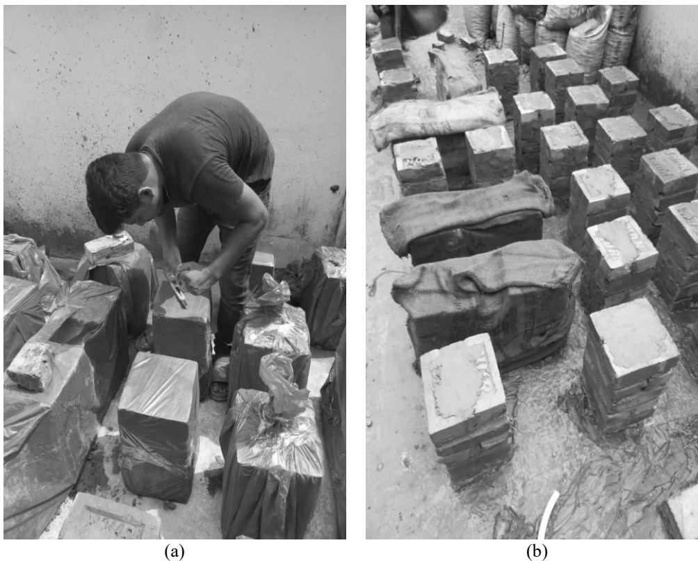
Figure 2: Brick masonry column: (a) Water-tight curing; (b) Wet gunny bag curing.
