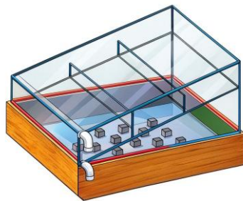
Figure 2: Single slope double basin solar still
