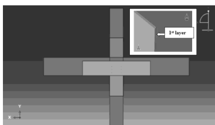
Figure 12: Retrofitted beam-column joint with one layer of TRM.
