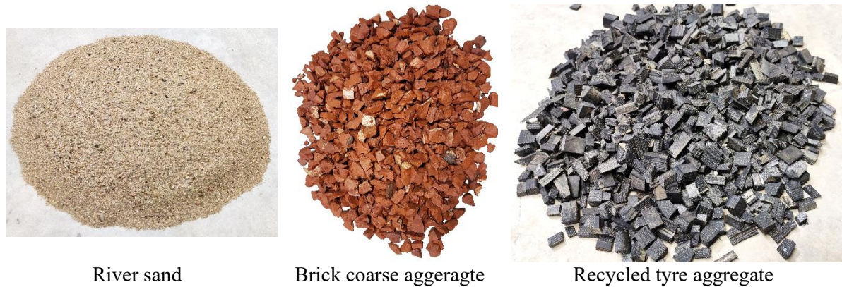
Figure 1: Images of river sand, brick coarse aggregate (BCA) and recycled tyre aggregate (RTA).
