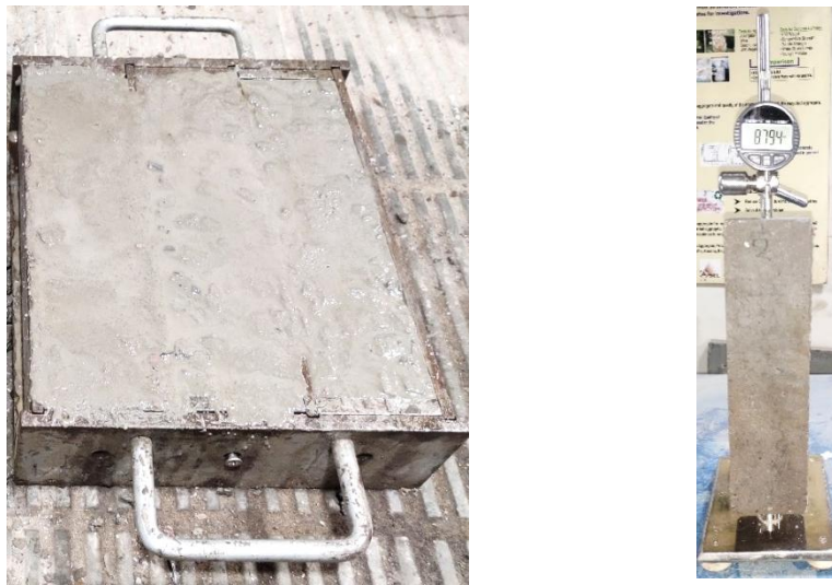
Figure 3: Fresh concrete with a prism for the shrinkage test (left) and prism specimens with a dial gauge to monitor the axial length change.
