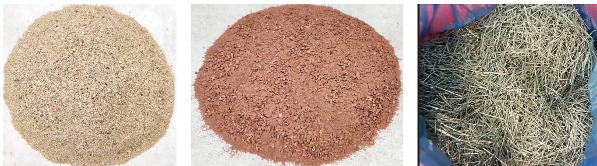
Figure 3: Image of sand (S), waste brick powder (WBP), and galvanised iron wire fibres (GIF).
