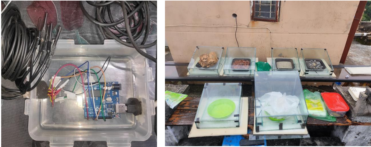
Figure 4: Arduino Uno board with temperature data logger & Six identical stationary water collection stills
