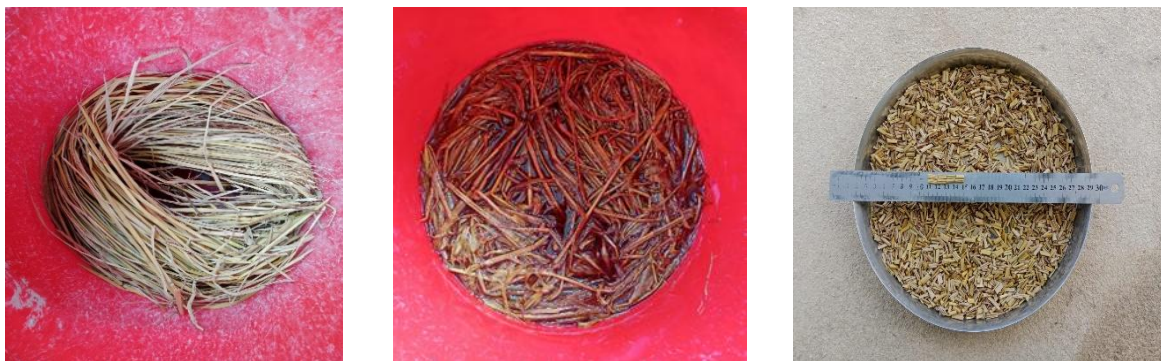
Figure 2: (a) Air-dried treated straw; (b) Alkali treatment of straw; (c) straw size (8-12) mm.
