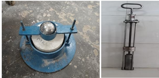
Figure13: Test Setup with Steel Ball and 4.5 kg Hammer
