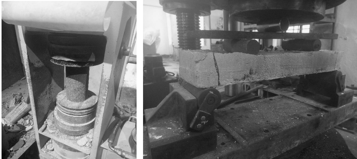
Fig 2.4.1: Conduction of Compression test and Flexural test using UTM
