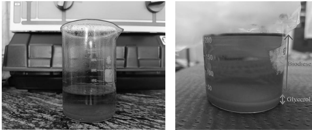
Figure 2: Visual appearance of biodiesel and glycerol layer
