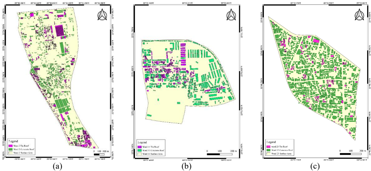
Figure 9: Measured Tin and Concrete Roof Area in Ward 2(a),11(b), and 23(c)
