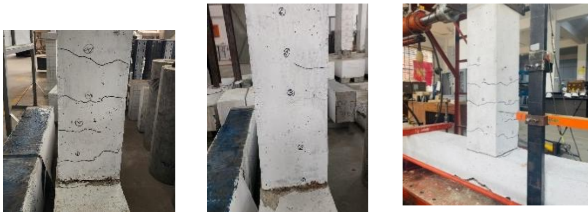
Figure 5: Cracks and failure zones of the beam-column joint in different locations.
