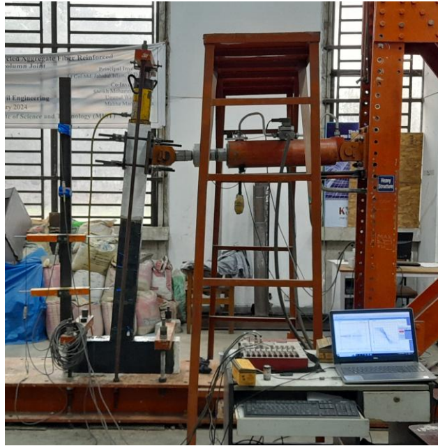
Figure 3: Cyclic loading test setup.
