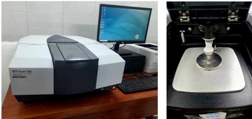
Figure 4: Shimadzu IRTracer-100 spectrometer (left) with ATR accessory (right)
