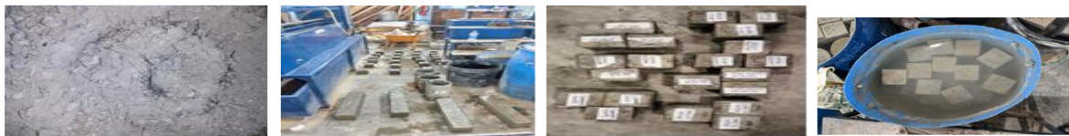
Figure 3: Concrete specimen preparation and curing at different coir and steel fiber dosages
