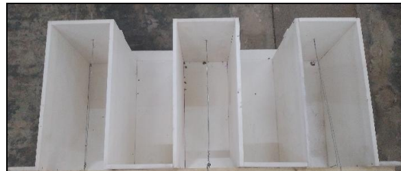
Figure 4: Schematic drawing and fabricated Rectangular Labyrinth Weir of three cycle
