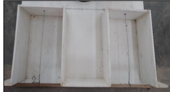
Figure 3: Schematic drawing and fabricated Rectangular Labyrinth Weir of two cycle
