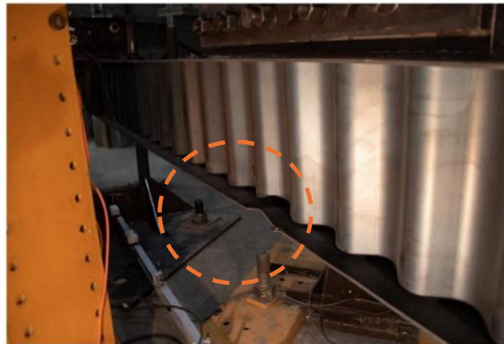
(b) Local Flange Buckling
