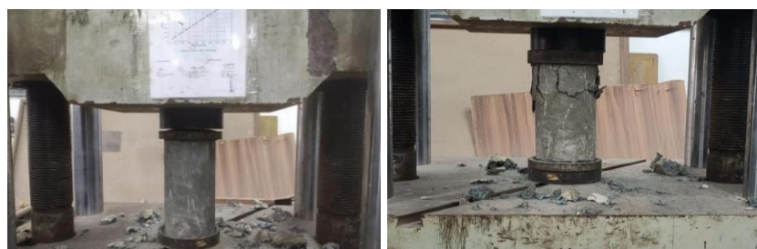
Figure 4 Compressive strength testing of concrete specimens.
