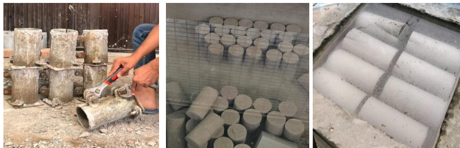
Figure 3 Casting and curing of cylindrical concrete specimens.
