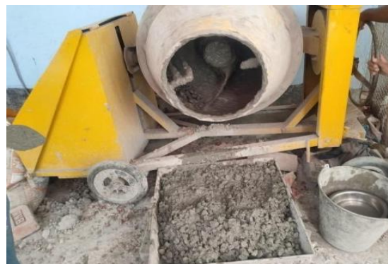
Figure 2 Mechanical mixing of concrete in the laboratory.
