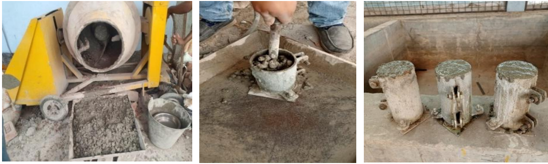
Figure 3 Casting and compaction of cylindrical concrete specimens.
