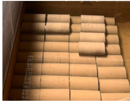
Figure 4 Water curing tank at DUET Civil Engineering Laboratory.
