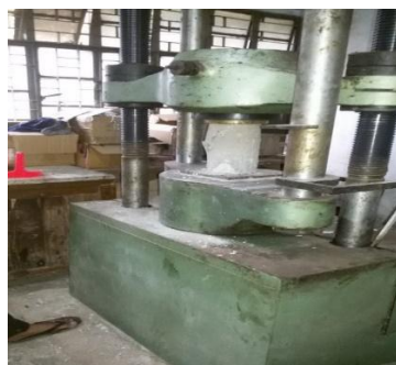
Figure 5 Compressive strength test setup.
