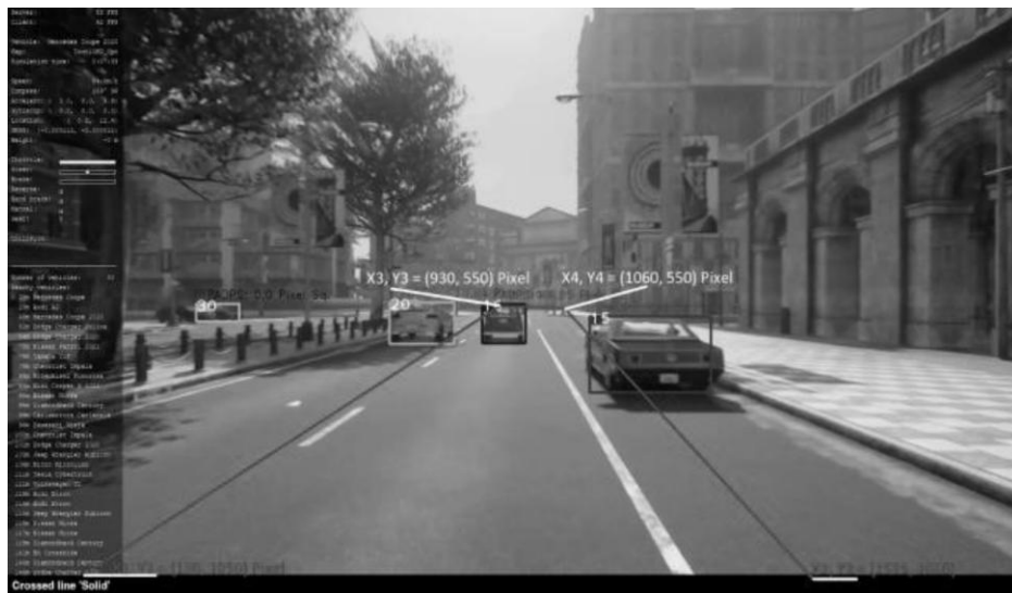
Figure 4 : Illustration of coordinates (specific pixel point in frame) identifying the critical section (X_1 = 150, Y_1 = 1050) , (X_2 = 1525, Y_2 = 1050) , (X_3 = 930, Y_3 = 550) , (X_4 = 1060, Y_4 = 550)
