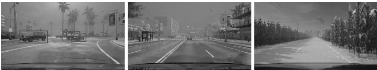
Figure 7: The left one illustrates the annotation of vehicles within 50 meters from the ego vehicle. The middle one illustrates ignoring vehicle annotations beyond 50 meters from the ego vehicle. The right one is an example of a zero-vehicle instance in the training dataset.
