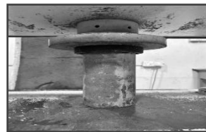
Figure 4: Compressive Strength Test
