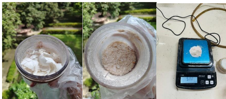
Figure 5. Eggshells were converted to powder, and 5gm powder was measured to add with sample.
