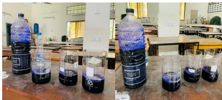
Figure 6. Samples were taken into 3 different beakers, and eggshells were added
