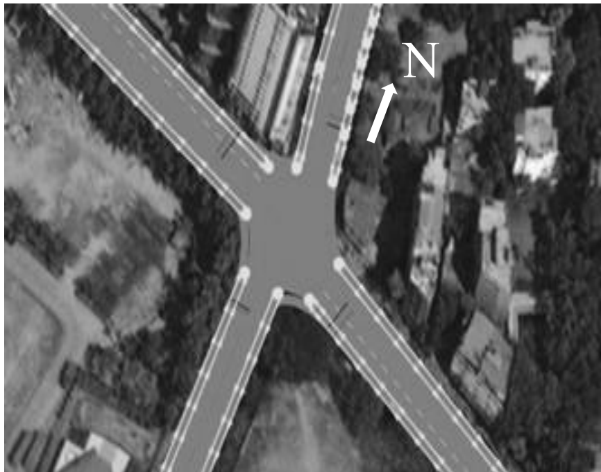
Fig 6: Modified Model having dedicated NMV Lane
