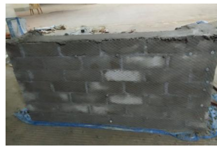
(b) Strengthening by Ferrocement lamination
